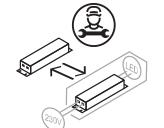
Replaceable control gear by a professional
