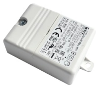
REQUIRED F990B34A000 Power Supply dual function C.V. Vout 24Vdc 8W, Vin 220÷240V C.C. Iout 350mA: 8W, Vin 220÷240V IP 20 Class II Selv. NON Dimmable
