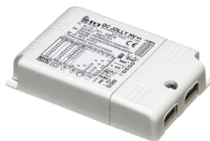
OPTIONAL Power supply FA135 Power supply 13 x 2W/ 110÷240V - Iout 500mA (7x2W@110V) IP20 Class II Selv. Eq. Dimmable Push- Dimm Or 1.10V
