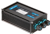
OPTIONAL Power supply FA218 Power supply 13 x 2W/ 110÷240V - Iout 500mA (7x2W@110V) IP67 Class II Selv. Dimmable Push- Dimm Or 1.10V
