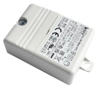
OPTIONAL F990B34A000 Power Supply dual function C.V. Vout 24Vdc 8W, Vin 220÷240V C.C. Iout 350mA: 8W, Vin 220÷240V IP 20 Class II Selv. NON Dimmable
