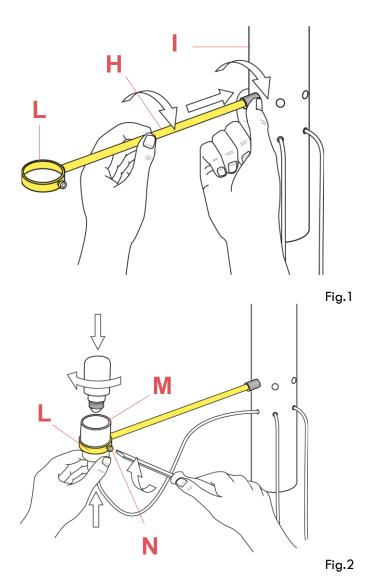
Screw the arms (H) to the lamp body (I), taking care not to bend on the rings (L). Insert the lamp holder (M) in the ring (L) and fasten them by locking the screw (N).
