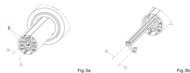
Fig. 3a - disconnect the terminal of the LED board that we need to replace (E).
