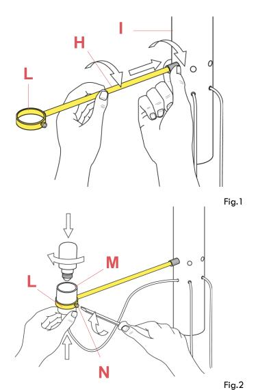
Screw the arms (H) to the lamp body (I), taking care not to bend on the rings (L). Insert the lamp holder (M) in the ring (L) and fasten them by locking the screw (N).
