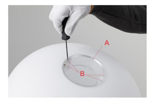
Insert the ring nut (A) in the glass diffuser hole and then fasten the screws (B). REMARKS!!! Do not tighten the screws hard. Risk cracking the glass diffuser.
